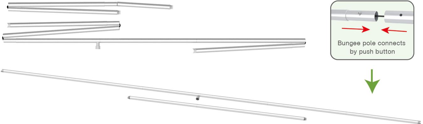
**STEP 05** To connect the bottom & top ring by using curved corner pieces according to labellings
