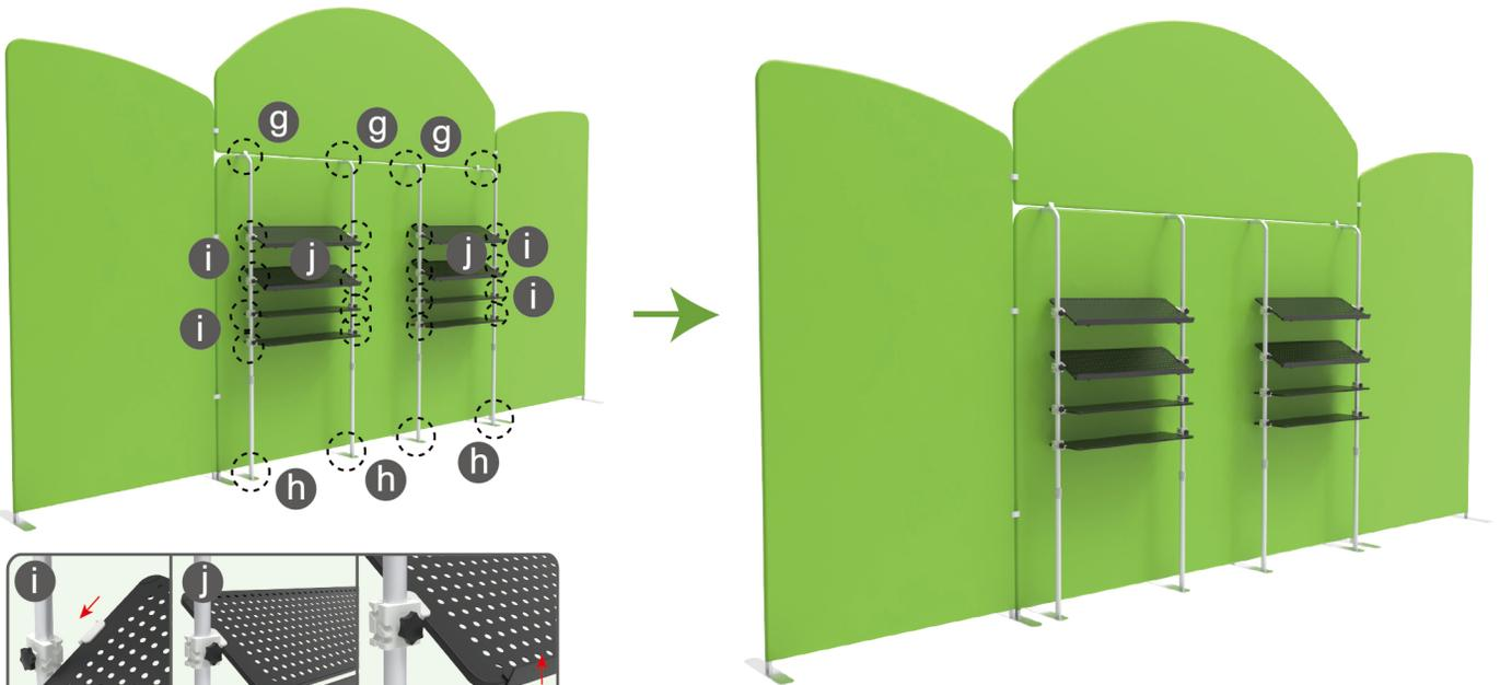
Clip into hanging boards based on directions of three-way clips & tightening with thumb screws, clip F-shaped bar onto hanging board with thumb screws.
