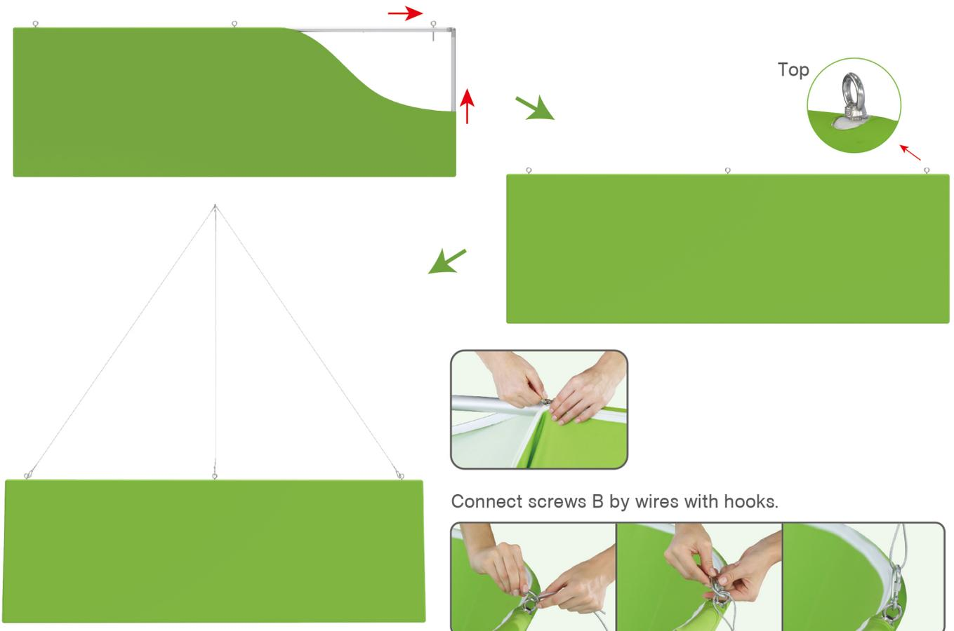
Connect screws B by wires with hooks.
