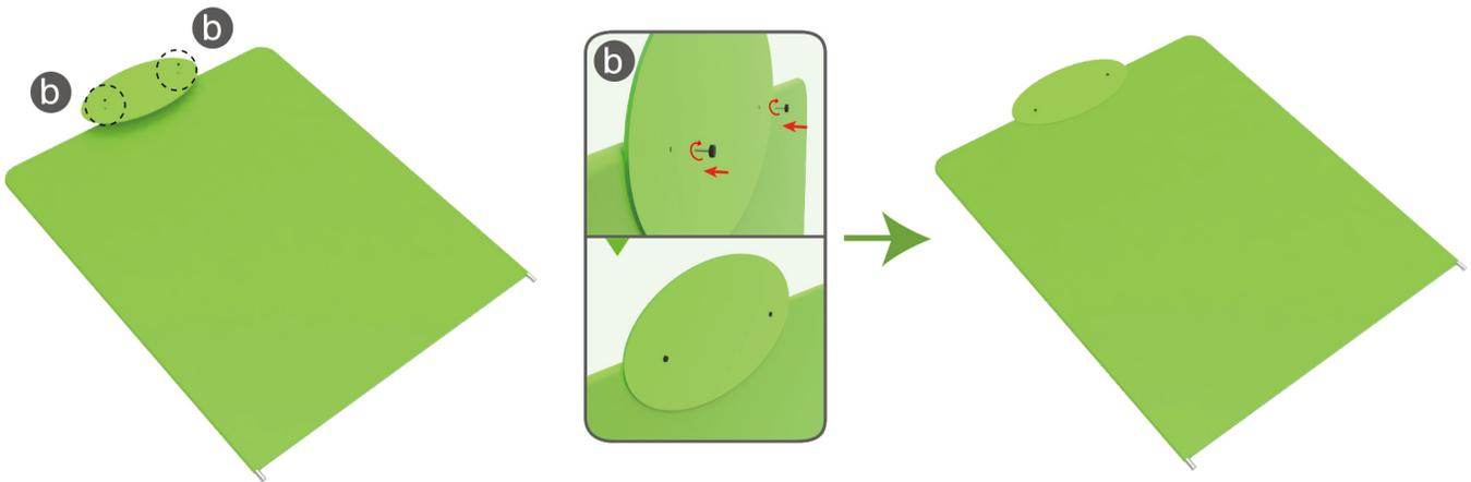
**STEP 02** Insert display stands onto feet by pressing their knobs.
