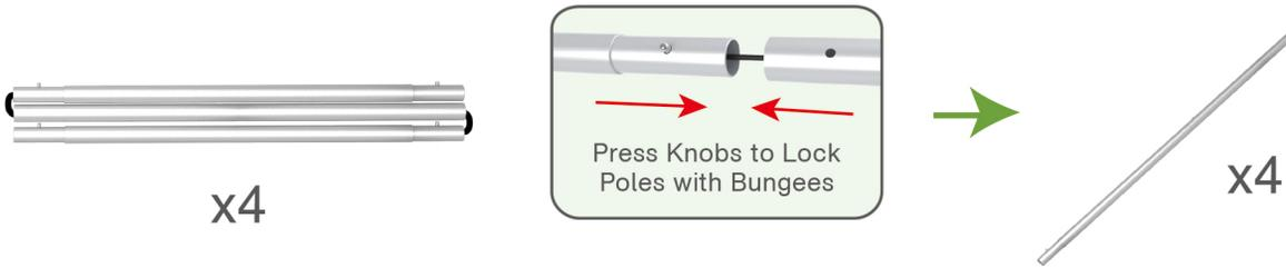
**STEP 02** Connect long poles with corner poles according to labelings.
