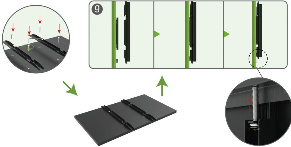
**STEP 06** Screw light clips at top of display stands, slide lights onto them and adjust their direction.
